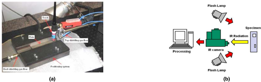
Fig. 6. Schematic description of the experimental setup used (a) to perform the TIG welds and (b) to record the thermographic image sequences.
